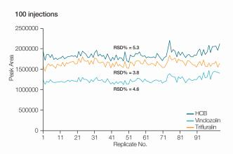
100 repeat injections of a tomato extract spiked at 10  $\mu$ g/Kg shows sensitivity is maintained over the 66 hours of continual operation.
