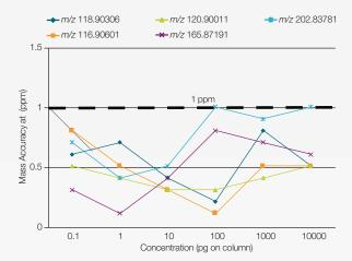
Mass accuracy of hexachloroethane ions <1 ppm over six orders of magnitude (0.1 to 10,000 pg. on column). High quality mass measurements are maintained for both trace and high concentration components.
