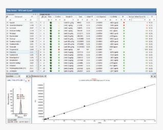
TraceFinder software uses the Exactive GC system data and combines compound detection, identification and quantitation to enable routine trace pesticide analysis to regulatory requirements. It also allows customizable, automated flagging for detected compounds along with flexible reporting tools.
