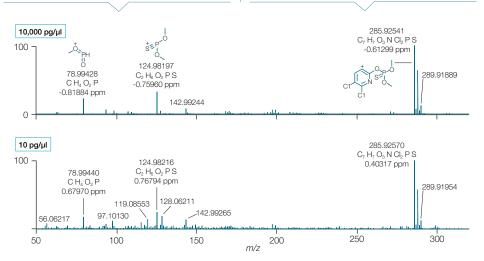
Full-scan spectra of chlorpyriphos-methyl at 10,000 and 10 pg/µl with fragment assignment using Thermo Scientific™ Mass Frontier™ software. Spectral fidelity and sub 1 ppm mass accuracy is maintained across the spectrum at both low and high concentrations.
