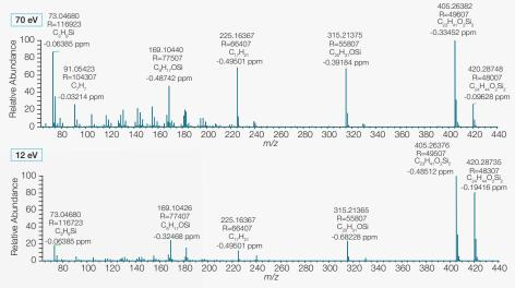
Epitestosterone shown with standard EI and VeV EI. Using VeV, the molecular ion signal and high mass fragment abundance are greatly increased, improving sensitivity for quantitative analysis and further MS/MS fragmentation experiments.
