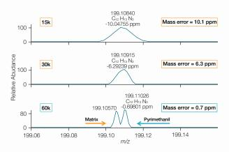
Impact of resolving power on the mass accuracy of Pyrimethanil at  $10 \mu g/Kg$  in leek acquired at different resolutions of 15k, 30k, and 60k. A resolution of 60k is required to resolve the Pyrimethanil ion from the matrix interference to achieve a mass accuracy compatible with the regulatory guidelines of <5ppm.
