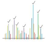
High-resolution filtering (HRF) algorithm uses accurate-mass information to discriminate against unlikely candidates based on elemental composition for every ion in the mass spectrum. This provides a high confidence identification of components detected.
