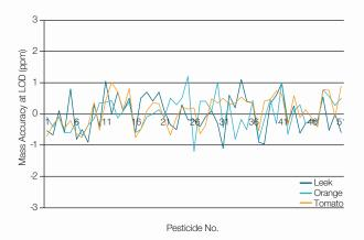
Mass accuracy at the limit of identification (0.5-5  $\mu$ g/Kg) for 51 pesticides in leek, orange and tomato matrices. The consistent low mass errors provides high confidence in positive identifications.
