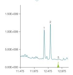
Accurate mass deconvolution extracts both high and trace level components to provide clean mass spectra and a comprehensive profile of a sample. Shown here are major peaks (1–2) in the TIC and a minor component in green (3).
