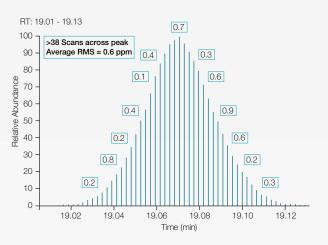
Extracted ion chromatogram of chlorobenzilate (m/z 251.0025 ±5 ppm mass window) in leek spiked at 10  $\mu$ g/Kg showing >38 scans/ peak (peak width 6 sec). Data acquired in full-scan at 60k FWHM resolving power. Excellent accurate mass (ppm) achieved for each individual scan (every third scan labeled). Average (RMS) mass difference of 0.6 ppm across the peak.
