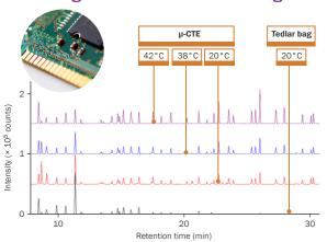
Quick investigations of how emission profiles vary under different conditions are easily conducted using the µ-CTE. This example shows the detection of residual solvents in **printed circuit boards**.
