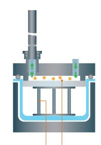
Sprung spacers raise planar samples to the top of the chamber.
