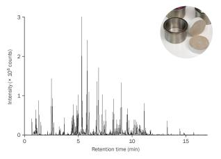
The µ-CTE is ideal for screening emissions from products such as flooring and plasterboard, for routine factory production control under the Construction Products Regulation (see prEN 16516).
