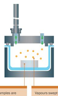
Samples are placed straight into the chambers.
