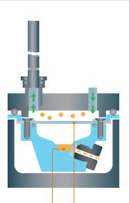
Liquid samples are injected through a septum into the well under a sealed sample of test material. Vapours diffuse through the test material into the chamber.
