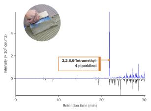
Emission profiles of similar products like these two brands of **grab-adhesive** are readily compared using the  $\mu$ -CTE – aiding product development and compliance with standard methodology such as ASTM D7706-11.
