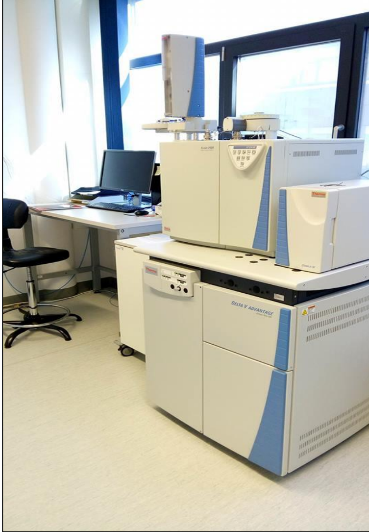
Thermo Scientific™ Flash™ 2000 Elemental Analyser connected to a Thermo Scientific™ DELTA™ V Isotope Ratio Mass Spectrometer http://serc.carleton.edu/research_education/geochemsheets/techniques/gassourcemassspec.html
