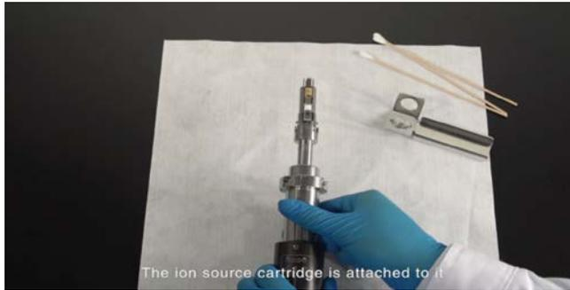
The ion source cartridge is attached to it
