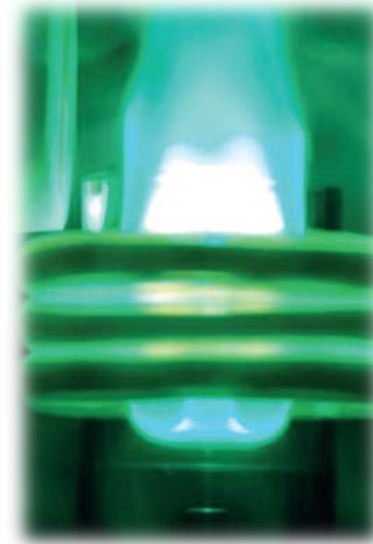
Plasma aspirating naphtha after auxiliary and nebulizer gas flows have been optimized.
