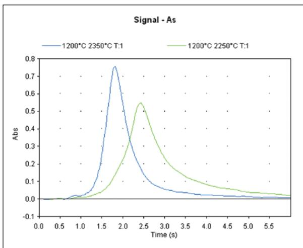
Figure 6: Arsenic signals at different Atomization Temperatures
