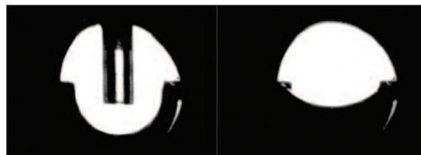
Figure 2: Optimized Capillary Tip position and Sample Injection
