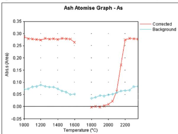
Figure 4: Automatic Ash Atomize plot for NIST 1640 water CRM
