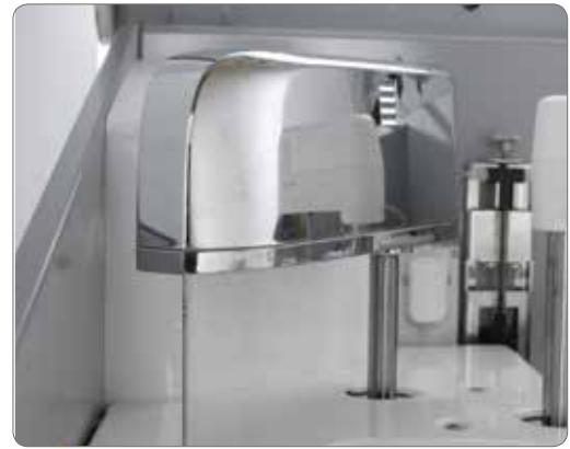
The Bitterness unit (BCM) in Gallery Plus Beermaster includes a coated capillary column for bitterness measurement.
