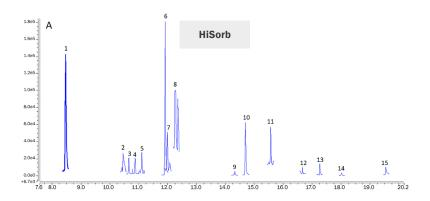
**Routine analysis of water samples** using different sampling techniques is achieved using the same Centri 180/GC-MS system: (Top) An 83-component mix of volatile organics by HS-trap; (Bottom) A suite of odorous compounds by HiSorb automated analysis. (See Markes' AN285) for details.)
