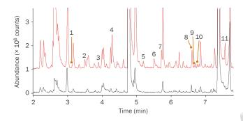
**Multi-step enrichment** (red trace,  $3 \times 5$  mL) greatly increases the number of important trace-level aroma compounds identified in this headspace-trap analysis of orange juice.
