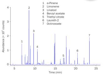
**Information about the semi-volatile components** in this fragranced shower gel is obtained using immersive high-capacity sorptive extraction. The large phase volume provides greater sampling capacity than SPME fibers, making it ideal for trace-level analysis.
