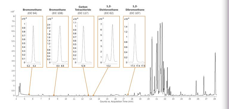
**Enhanced sensitivity and excellent peak shapes** are achieved for the detection of early-eluting, trace-level volatile fumigants (at 0.005 mg/kg), in this ground pepper sample. Sizeable improvements in the signal-to-noise ratios are obtained when combining Centri 90 with GC-MS.
