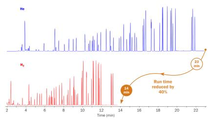
**Analysis of 'air toxics' at ppt to ppm levels:** Using hydrogen as a carrier gas it is possible to significantly reduce the run time while still maintaining excellent separation.
