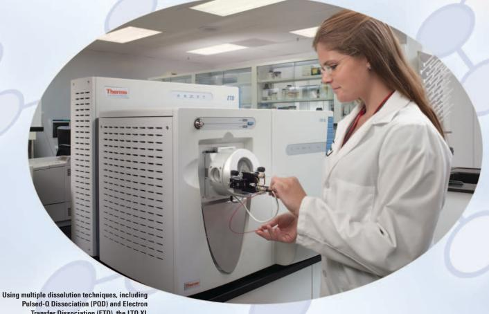
sing multiple dissolution techniques, including Pulsed-Q Dissociation (PQD) and Electron Transfer Dissociation (ETD), the LTQ XL generates extensive structural information for the most demanding proteomics samples.
