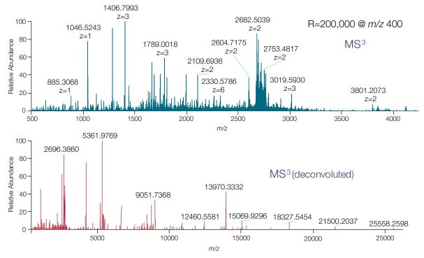
Q Exactive UHMR quadrupole selection of the monomer (shown at the bottom of the previous page), followed by fragmentation in the HCD cell for pseudo-MS³ analysis.
