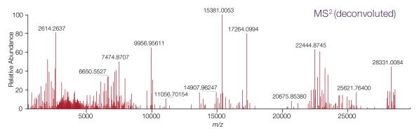
Native top-down analysis of the AmtB membrane protein complex enabled by high mass quadrupole selection and efficient HCD fragmentation.
