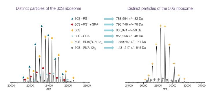
High-resolution MS data produced by the Q Exactive UHMR mass spectrometer reveals the heterogeneity of the ribosomal particles and the substoichiometric association of stationary phase-induced ribosomal-associated protein (SRA).
