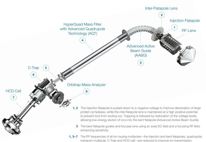
High mass ions are efficiently injected into the Orbitrap mass analyzer by adjusting the slew
