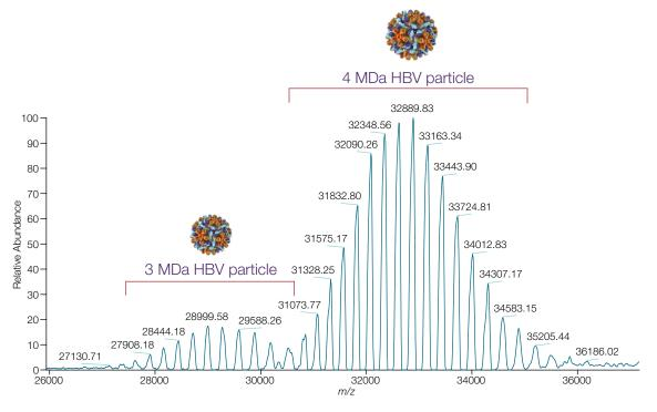
Mixtures of 3 MDa and 4 MDa hepatitis B virus capsids analyzed under charge reducing conditions span a wide mass range between 27,000 and 36,000 *m/z*. The spectrum contains well-resolved charge states for both particles and shows no bias for the 25% smaller 3 MDa particle.
