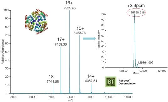
In-source trapping allowed efficient removal of detergent micelles for accurate native MS analysis.
