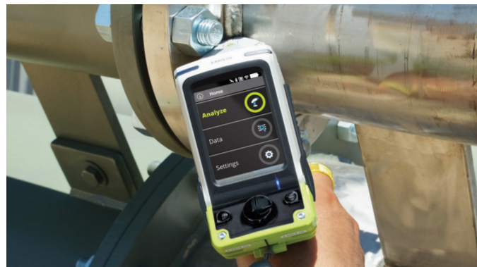
The Niton XL5 Plus in use, analyzing a tight weld in an oil refinery.
