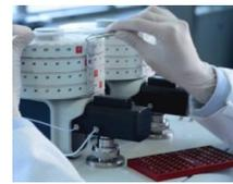
Introduce the sample into the MAS Plus Autosampler
