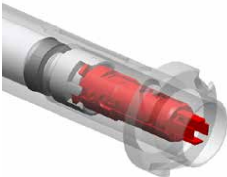
Step 3. Hot source is held in tool
